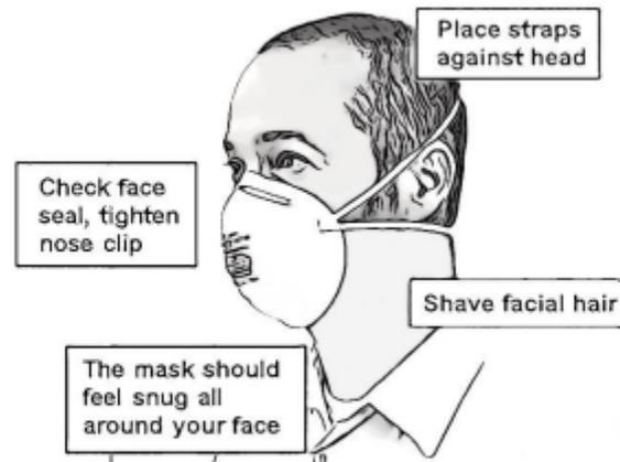
*Drawing Showing Proper Fitting of a Filtering Facepiece Respirator
